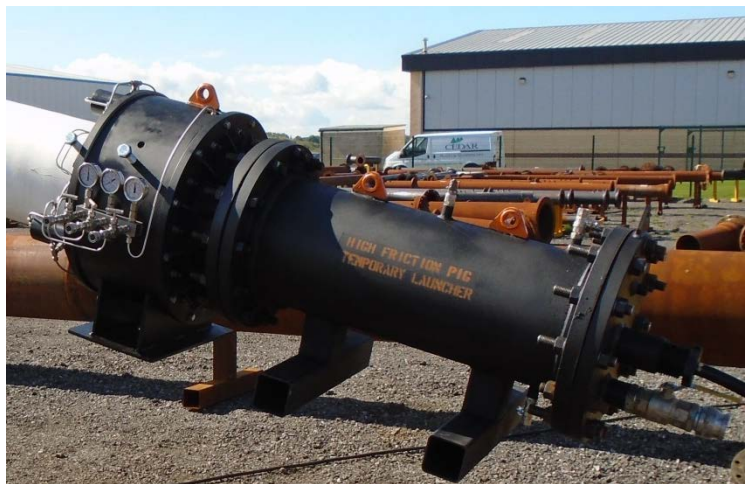
A 14" NS External Pipe Plug c/w Temporary Pig Launcher
