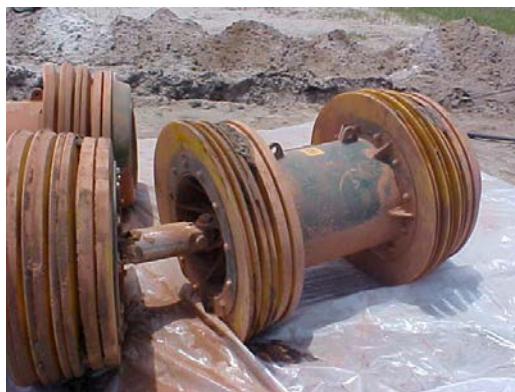
Fig. 7 – Pig condition, post run
