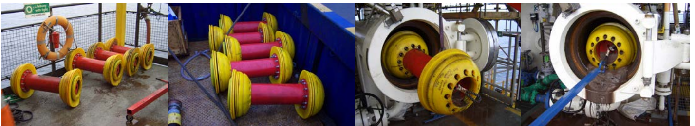
(Figure.1. 20"ns Uni-Di pig traversing check valve in reverse)
