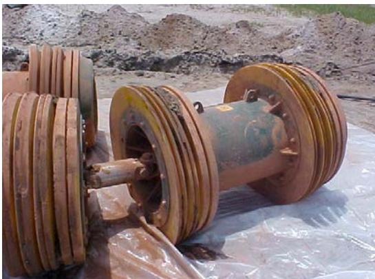
Pig condition after dewatering run
