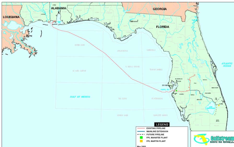
The Gulfstream pipeline is the largest pipeline in the Gulf of Mexico. It was also the first new natural gas transportation system to serve Florida in more than 40 years. The system is expected to supply Florida with approximately 1.1 billion cubic feet of natural gas per day.
